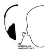
Figure 7: Coupling a hearing aid to an ALS by placing the headphone over the hearing aid while it is switched to the "T" setting.
