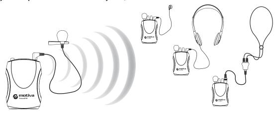
The speaker wears the belt-clip transmitter and a clip-on microphone. The speaker's voice is broadcast as an FM radio signal over a distance of 150 feet. Listeners use the pocket receiver and earphones or headphones to hear the speaker's voice directly, with reduced background noise. An optional neckloop telecoil coupler allows the system to be used with telecoil (T-switch) equipped hearing aids.
