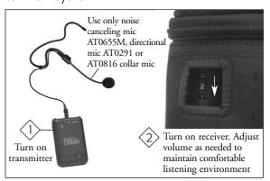
using 572R and 575R (requires AT0799 adapter) installation and operation for 572R/575R
